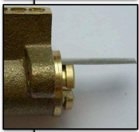
ONCE COMPLETED, YOUR SHIM WILL BE FULLY INSERTED INTO THE LOCK AND ALL THE DRIVER PINS WILL BE STUCK ABOVE THE SHEAR LINE. YOU ARE NOW ABLE TO REMOVE THE PLUG, BUT DON'T DO THAT YET! SEE THE NEXT PAGE FIRST!
