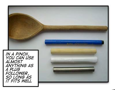
IN ORDER TO REMOVE THE PLUG, YOU WILL NEED A PLUG FOLLOWER. THESE CAN BE PURCHASED, OR MADE FROM WOODEN DOWEL. THERE ARE A VARIETY OF PLUG DIAMETERS, SO YOU WILL NEED A VARIETY OF PLUG FOLLOWERS. HOWEVER, THE MOST COMMON SIZE FOR LOCKS IN NORTH AMERICA IS 1/2 INCH.
