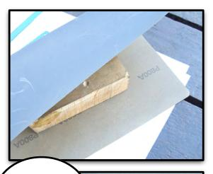
TO START, LAY THE PICK FLAT ON A SURFACE AND SAND. PICK FINISHING IS WHERE IT'S AT. GET GOOD AT THIS! THE SMOOTHER YOUR PICKS, THE EASIER THEY WILL MOVE THROUGH THE LOCK, THE BETTER FEEDBACK YOU'LL GET FROM THE PINS, AND THE BETTER YOU'LL BE AT PICKING LOCKS!
